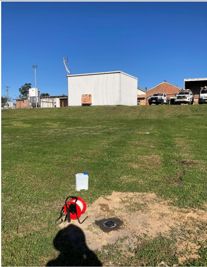
Groundwater Monitoring Well installed downgradient of the Yard Maintenance Shed
